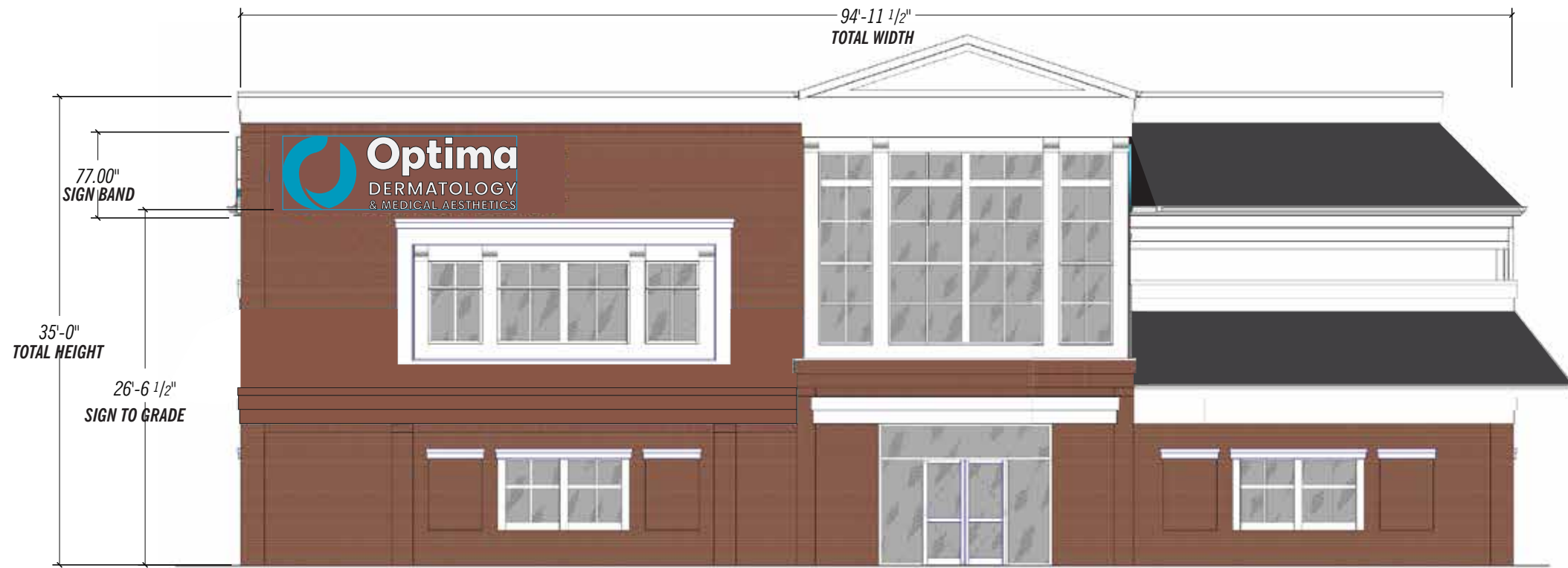
SIGN INSTALL - EAST ELEVATION
